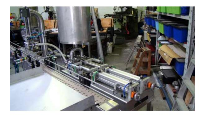
Pavar Automatic Volumetric filling machines are versatile and easy to operate.
